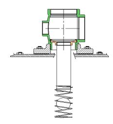
The float vent valve must be installed in vertical position on the manhole lid. For its installation it is possible to use extractor fitting Model 1531.
